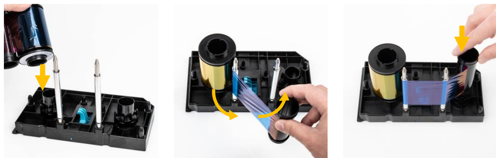
Figure 13 Loading the ribbon
