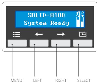
There is an LCD and 4 buttons on the front side of the SOLID-810. Users can check the printer status and change various printer settings.
