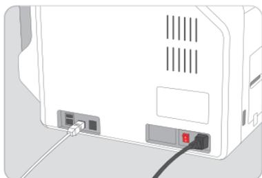
17. Connect the AC Power cable and USB cable.
