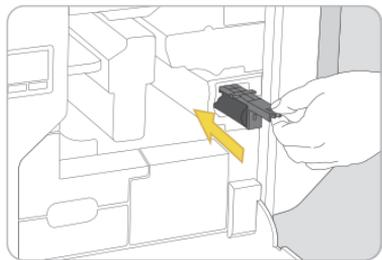
11. Mount the Disposable cleaning roller inside the printer.
