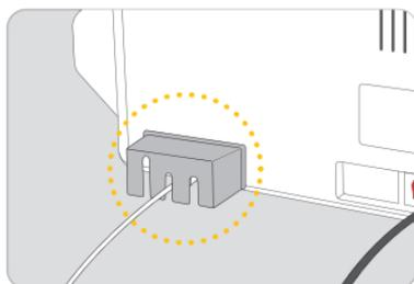
18. Install the Cable Protection Cover.
