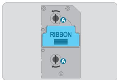
5. Insert the ① ribbon SUPPLY core on the mounting place of the cartridge core until it "clicks". Wind the ribbon around two shafts following the diagram arrow, and insert ② TAKE UP core into the core mounting until it "clicks".
