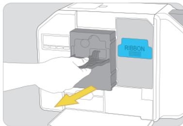
2. Hold the Retransfer film cartridge handle and pull it out.
