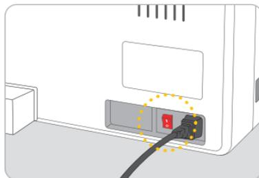
6. Connect the USB cable to PC and turn on the printer by pressing the On/Off button at the indicated point.
