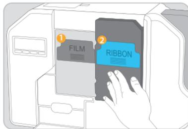
12. Mount ① Retransfer film cartridge at first and then, mount ② Ribbon cartridge.
