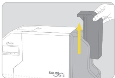
14. Open the Input Hopper cover in the direction of the arrow.
