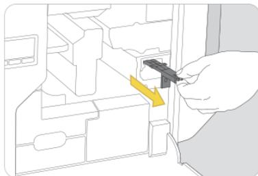
4. Hold the disposable cleaning roller cartridge handle and take it out.
