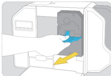
3. Hold the Ribbon cartridge handle and pull it out.
